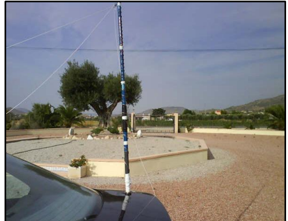
Close-up of the antenna mounting. The antenna is basically self supporting and can be used like this when the weather conditions are calm.
