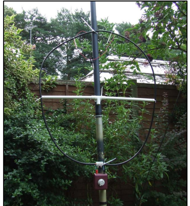
Quick and simple way to install the loop as a manually tuned or fixed frequency auxiliary antenna
